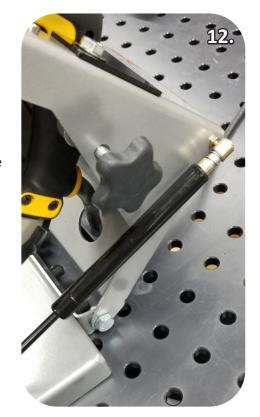
**12.** Reconnect the gas shock to the pivot ball on the top arm. The saw is now ready to plug in and perform test cuts.
