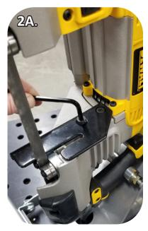
**3.** Install the Portaband table accessory using the DeWalt supplied hardware and wrench.
