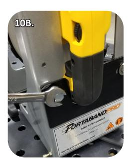
**11.** Using the included 3/32" hex key and an 11/32" wrench, reinstall the yellow trigger arm as shown.
