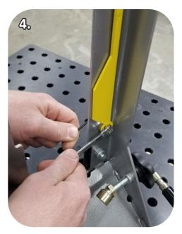
**4.** Using the included 3/32" hex key, and an 11/32" wrench, remove the yellow trigger arm and hardware from under the top of the jig. Save for reinstallation in step 11.
